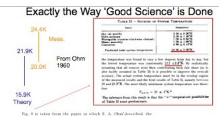
receiver on the 20-5oot horn reflector which was used to receive signals bounced from the Echo satellite. He found that its system temperature was 3.3. K higher than especied from summing the contributions of the components. As in the previous 5.3 cm work, this excess temperature was smaller than the experimental errors, so not much attention was paid to it. In
